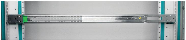
Fasten the rail on the rear side by using one deep-drawn washer and one countersink Phillips screw M5 x 10mm per rail.
