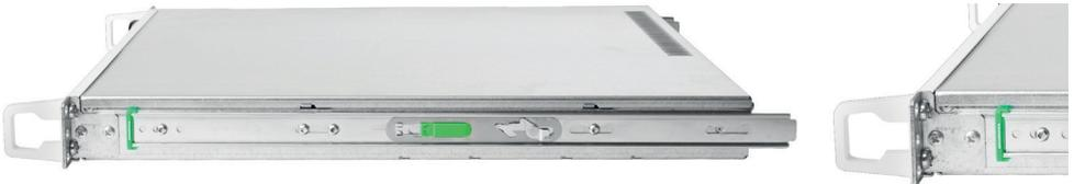
Short chassis – long rails: 4 screws per rail
