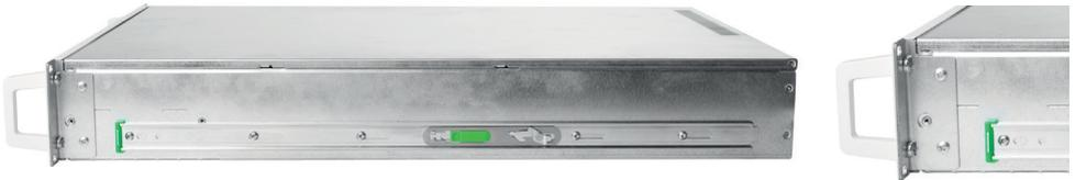
Short chassis – short rails: 4 screws per rail
