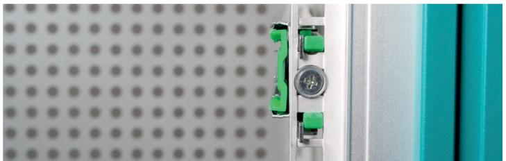
1U front: leave screw hole blank, as this is need for chassis locking
