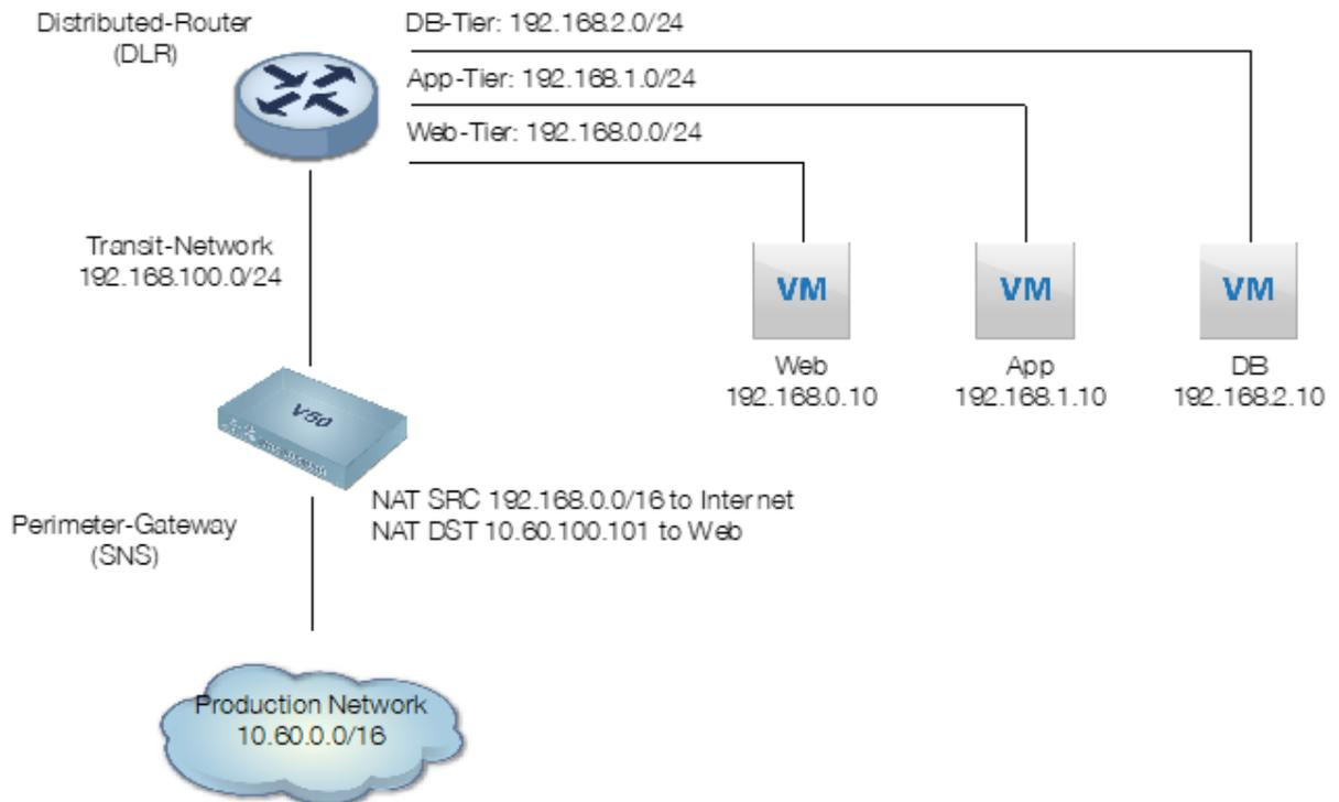
Setting up this architecture requires a virtual SNS firewall deployed on the platform with two interfaces taken out of the bridge created by default:
