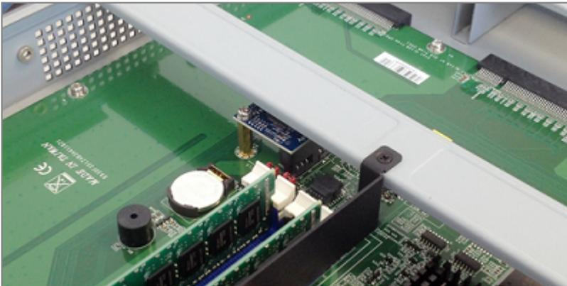
4. Unscrew the fastening screw of the Flash module with a Philips screwdriver, by keeping the associated hex spacer in place with a flat wrench:
