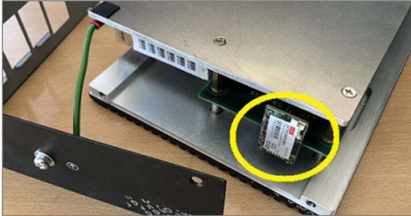
7. Unscrew the 5 silver fastening screws from the metal plate.
