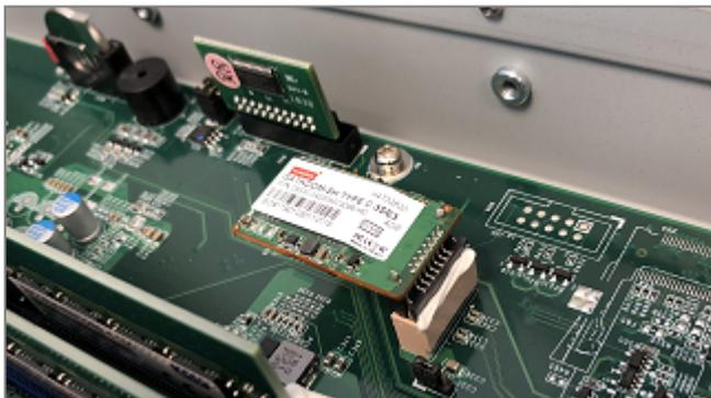
4. To extract the flash module, pull it gently and perpendicular to the motherboard:
