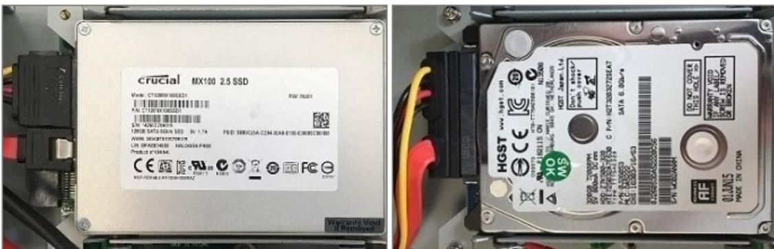
6. Unscrew the 4 fastening screws of the hard disk with a Philips screwdriver.
