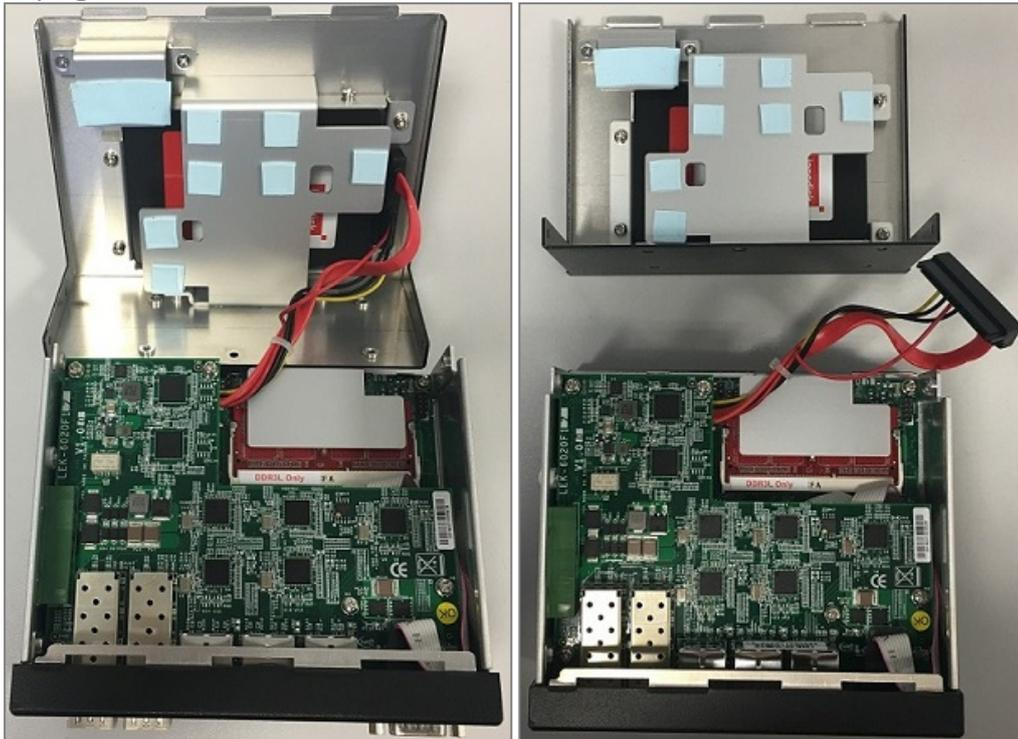
7. Unscrew the fastening screws from the hard disk support:
