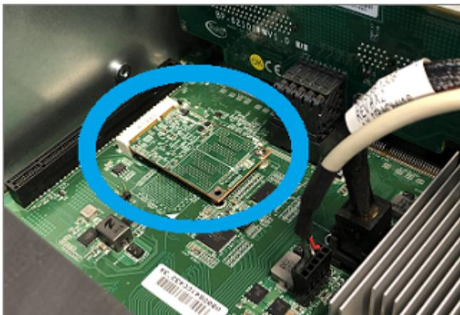
4. The flash module is fastened with one screw; remove it.
