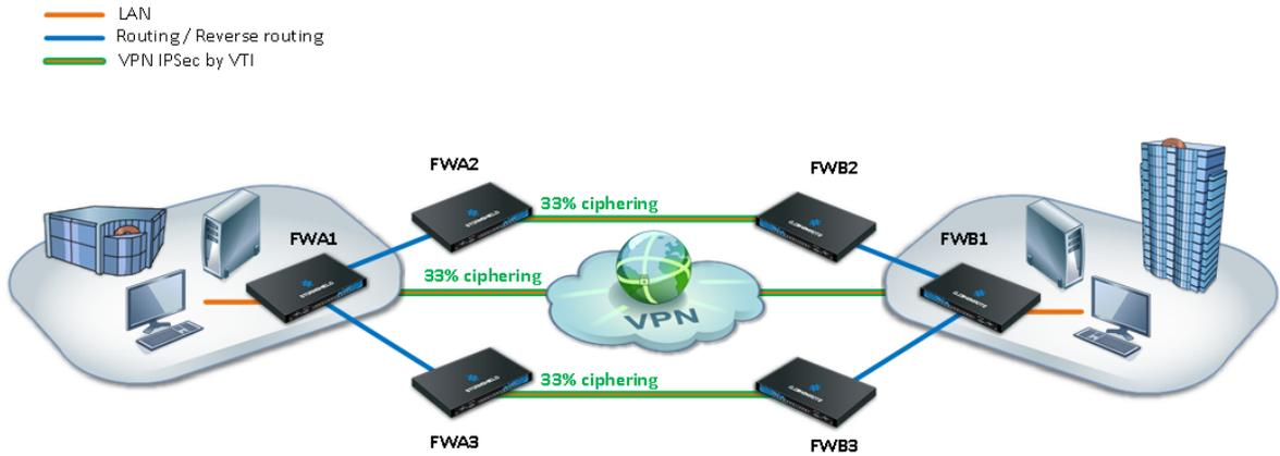
The first scenario shown in this technical note uses router objects and return routes in order to distribute IPsec tunnels over several firewalls, thereby spreading out the system resources needed for encrypting/decrypting data.
