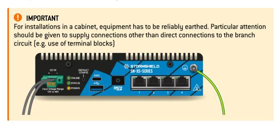
Once your firewall has been powered up, it will automatically start up. Wait for several minutes until the *Status* LED lights up.
