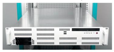
Pull each slider to the front and push the chassis completely into the rack.
