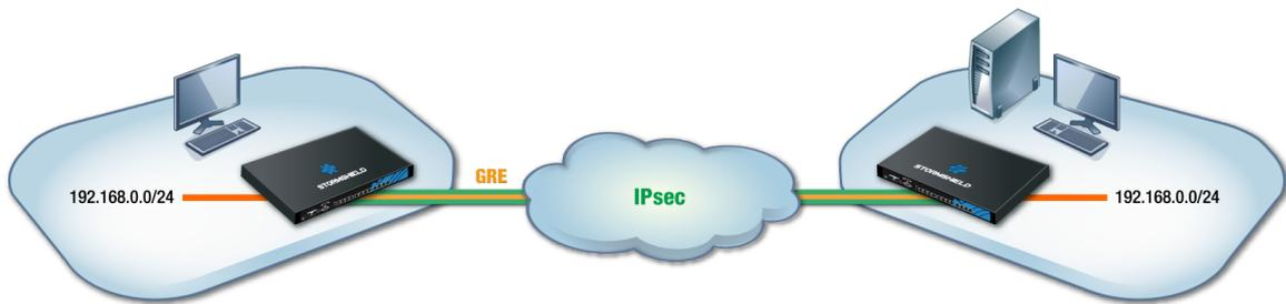
This section of the technical note sets out the scenario of a company seeking to link two sites sharing an identical address range through a bridge. Services, for example DHCP, and shared network resources will therefore be considered local services, regardless of the site. To secure exchanges, GRE traffic will be encrypted in an IPsec tunnel.
