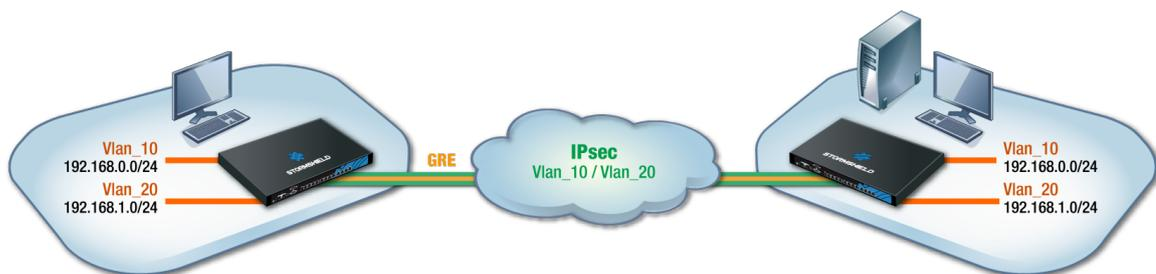
This section of the technical note sets out the scenario of a company seeking to share two VLANs between two sites through a GRE tunnel secured by encryption (IPSec). It covers the specific configurations in the creation of GRETAP interfaces, IPSec tunnels, VLAN settings and their attachment to GRETAP interfaces.
