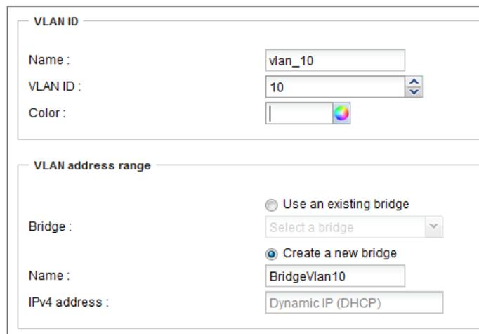
The screenshot shows a configuration window for a VLAN. It is divided into two sections: 'VLAN ID' and 'VLAN address range'.
