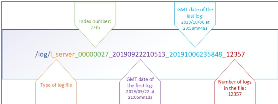
File indexation (managed incrementally and starting from 0) makes it possible to not have to rely only on creation or closing dates, as these dates may be distorted when the time is changed on the firewall.
