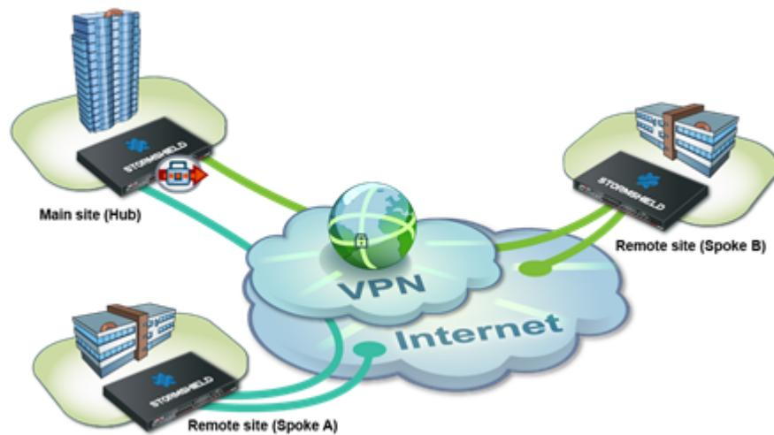
For the configuration of a Hub & Spoke IPSec policy, please refer to the *HOW TO* mentioned below. In our case, the differences from this procedure consist of configuring traffic endpoints through virtual interfaces, instead of remote networks in the IPSec policy (see following paragraph).
