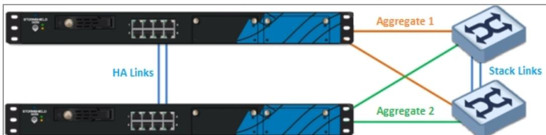
Two Stormshield Network firewalls form a high availability cluster with an active node and a passive node.
